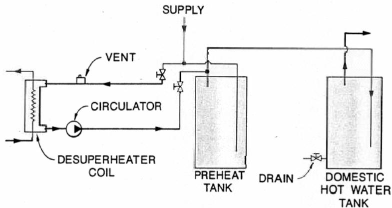
Figure 2.6 – Desuperheater Two-Tank System
