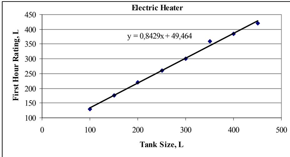
Figure 3.2 – First Hour Rating Relationship for Residential Water Heaters
