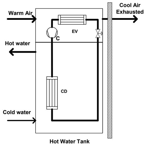
Figure 2.2 – Residential exhaust-air hot water heat pump
