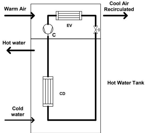
Figure 2.1 – Ambient air-source heat pump water heater
