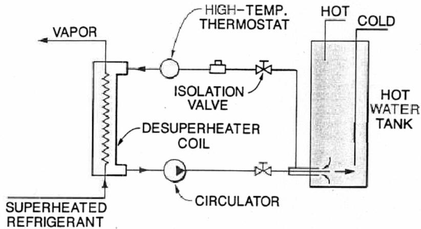
Figure 2.5 - Desuperheater System Configuration
