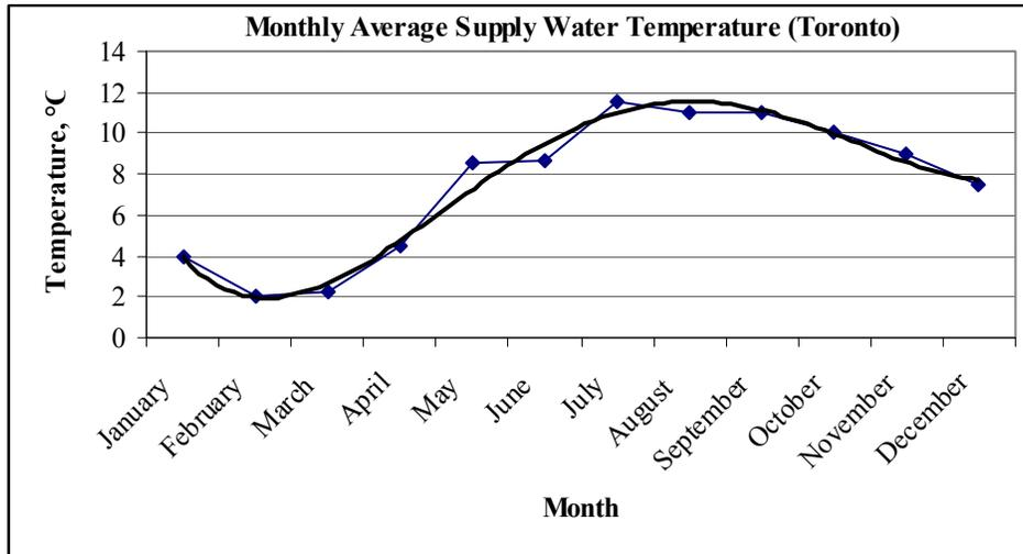
Figure 3.1 – Annual Variation of the Cold Water Supply Temperature in Toronto
