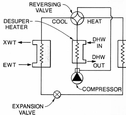
Figure 2.4 – Recommended Desuperheater Placement
