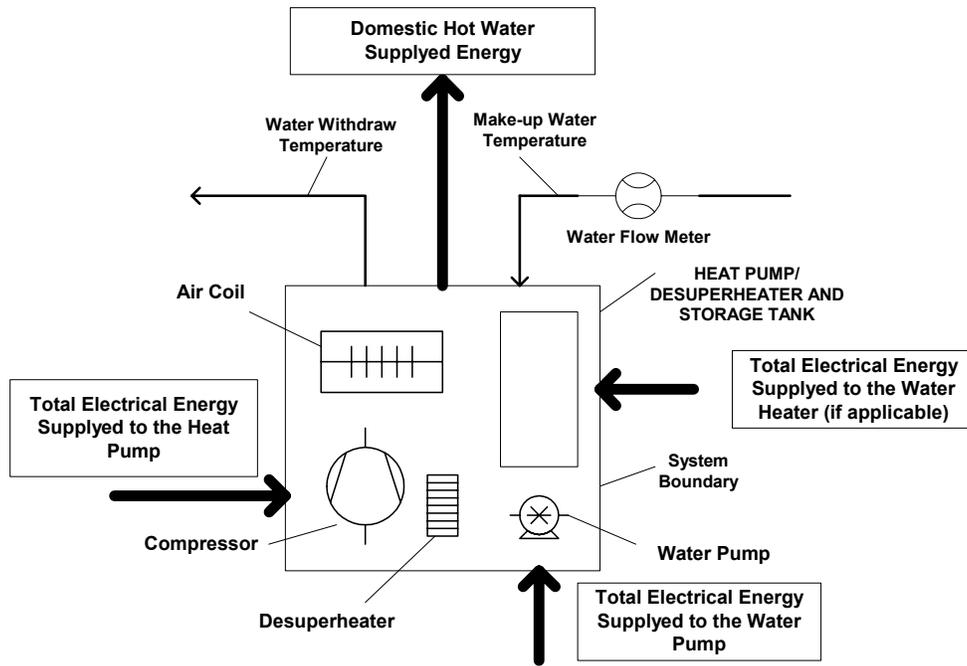
Figure 4.6 – Boundary Energy Conditions for a Combined Space and DWH Heat Pump with Desuperheater
