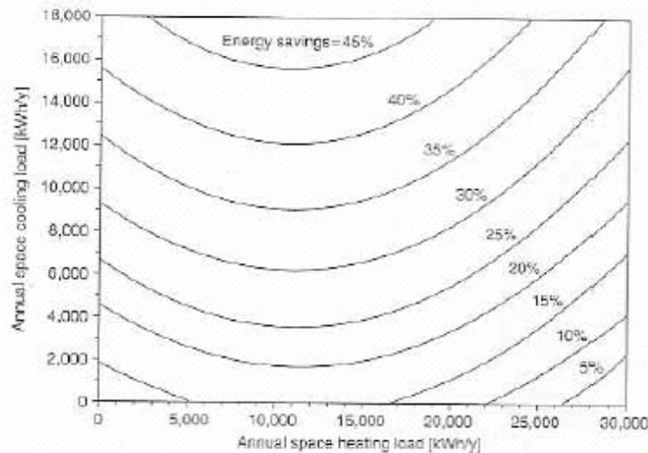
Figure 2.7 – Water heating energy savings with a desuperheater
