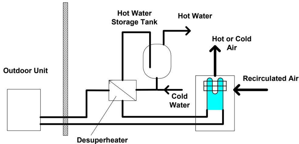
Figure 2.3 - Combined Space Heating or Air Cooling, and Hot Water Heating Heat Pump
